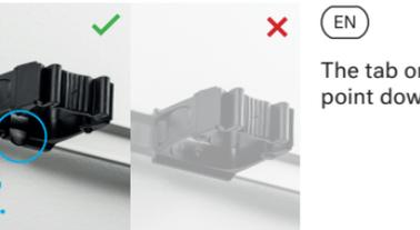
6. Install the holder by hooking the top at a 45° angle. Press until a click is heard.
